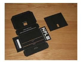
Cut out the main body of the spectrograph along the solid white lines, making sure to cut out the viewing window and either the CD or DVD ports. Cut out the entrance slit, keeping it as narrow as possible. (A craft knife is useful here, but ask an adult for help!)
