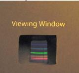
Point the slit at a light source and look through the viewing window at the CD. Looking slightly upwards towards the top of the CD you should clearly see a spectrum, the light split into its constituent colours.
