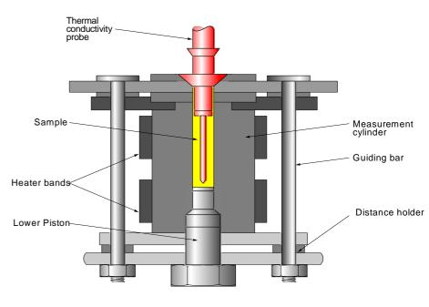
Measures thermal conductivity at industrially relevant processing pressures and temperatures
