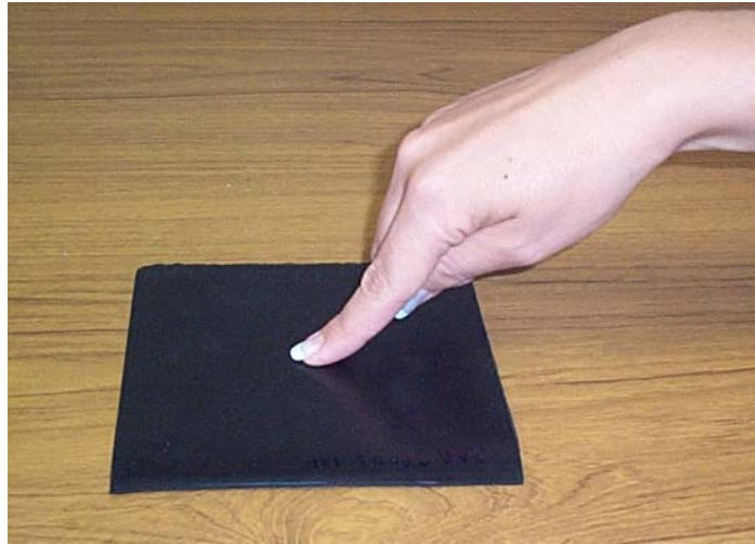
Figure 2: Procedure to assess the softness of a flat sample
