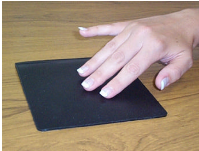
Figure 5: Procedure to assess the smoothness of a flat sample
