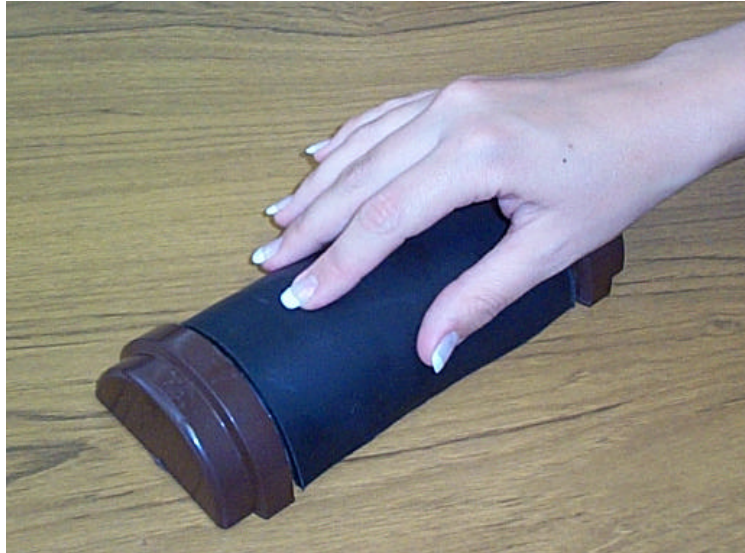
Figure 4: Procedure to assess the softness of a curved sample
