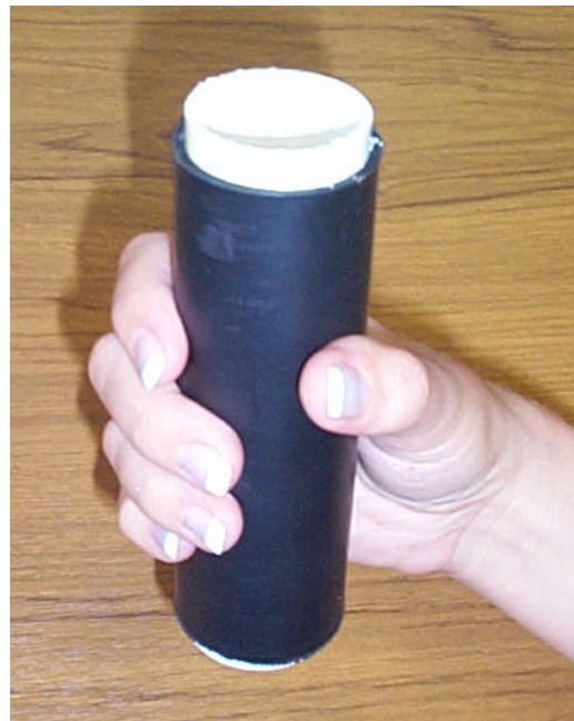
Figure 3: Procedure to assess the softness of a cylindrical sample
