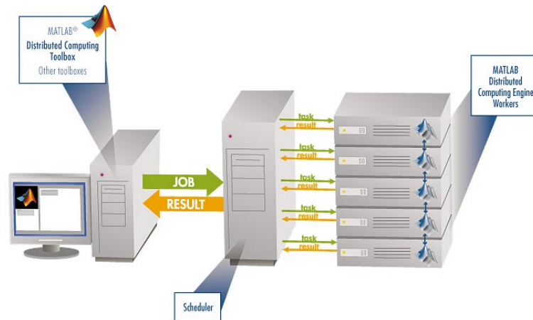
Figure E.1: The interaction between the client machine, where the Distributed Computing Toolbox is used to define jobs and tasks, and the MATLAB Distributed Computing Engine. The scheduler can be the MathWorks job manager, provided as part of the MATLAB Distributed Computing Engine, or a third-party scheduler.
