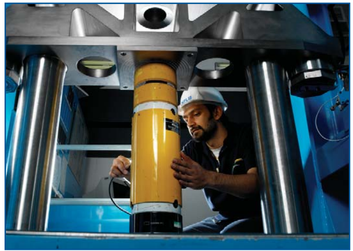
Calibrating a 4.5 MN force transducer in NPL's 1.2 MN deadweight machine
