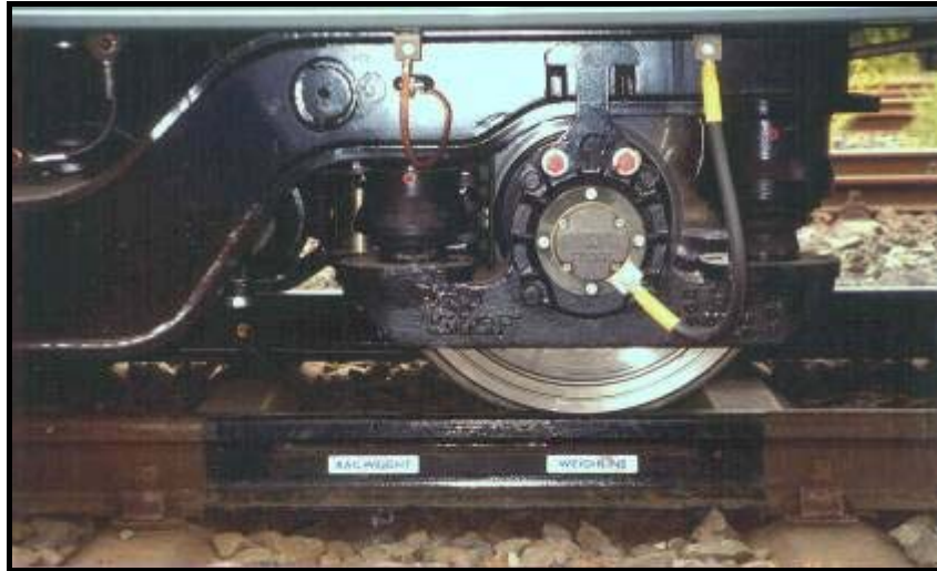
Figure 5.2.2.5 In-track weigh section
