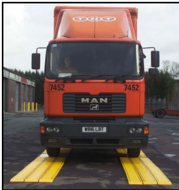
Figure 5.2.1.3 Surface mounted weigh pads with infill strips
