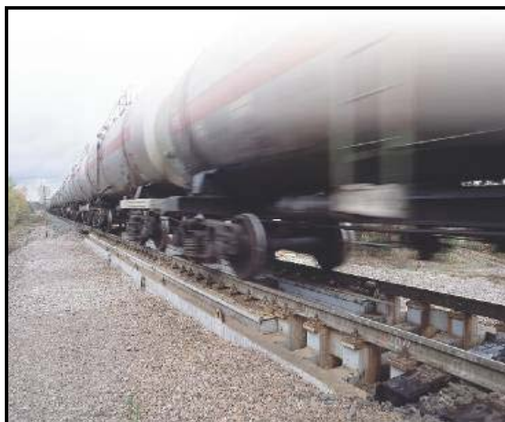
Figure 5.2.2.8 Surface mount weighbridge
