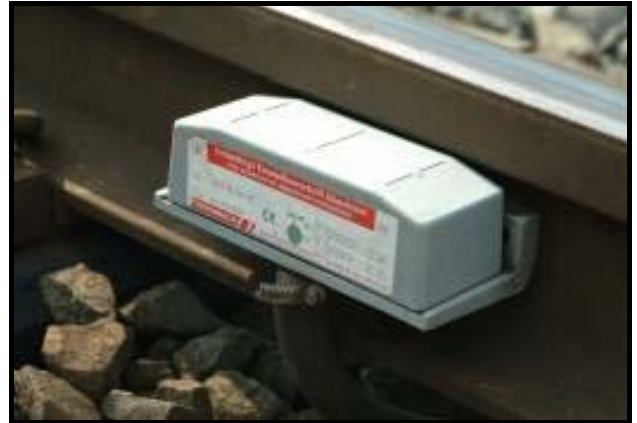
Figure 5.2.2.2 Inductive sensor wheel detector
