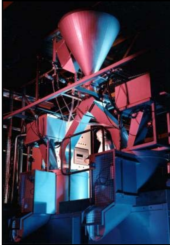
Figure 3.1.3 Typical process batch weighing system
