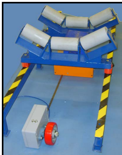
Figure 5.1.1.2 Belt weigher with two idler weighing mechanism
