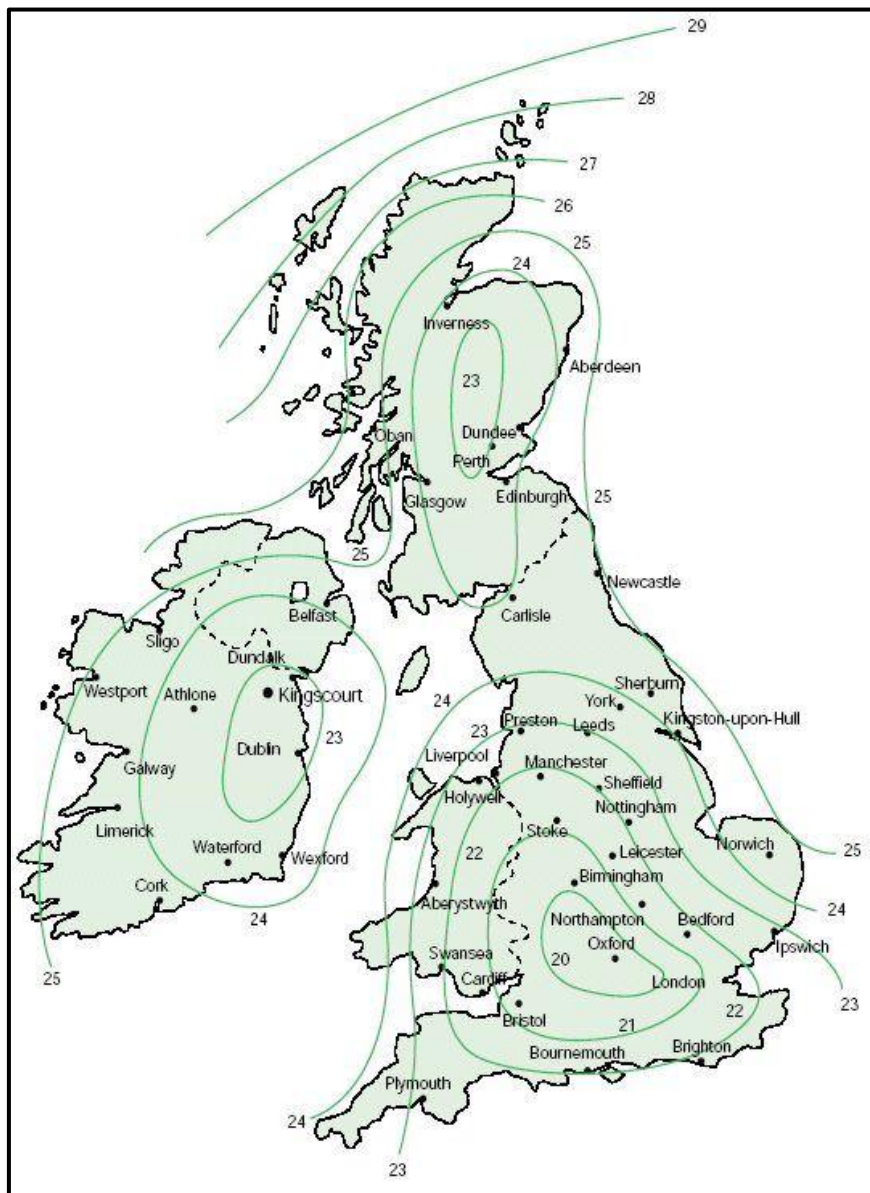
Figure 5.5.3 Basic wind speeds, in m \cdot s^{-1} , in the United Kingdom. This extract from BS 6399 : Part 2 : 1997 (now superseded by [12]), is reproduced with the permission of BSI
