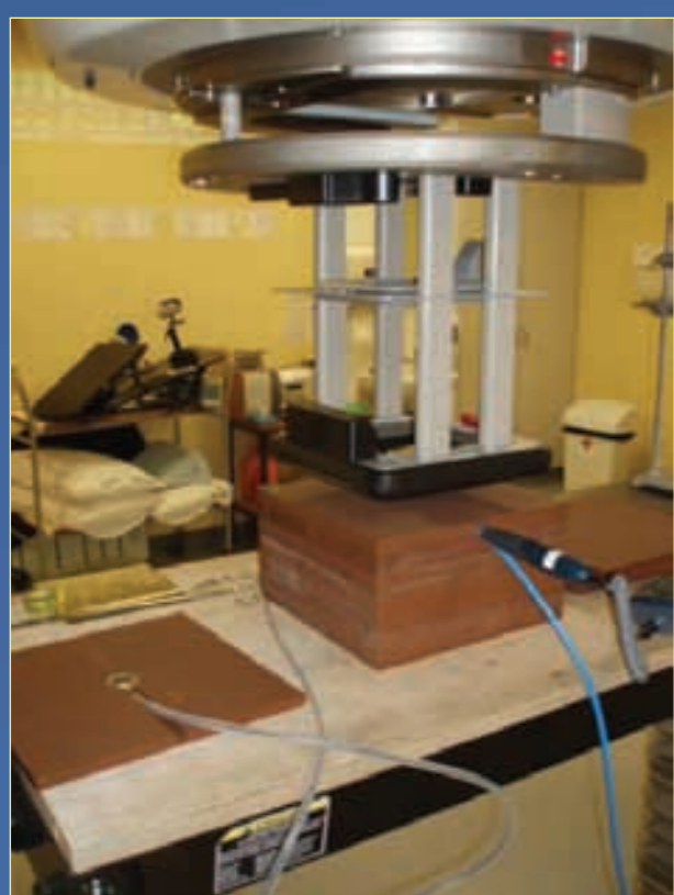
Electron beam output measurements in solid water
