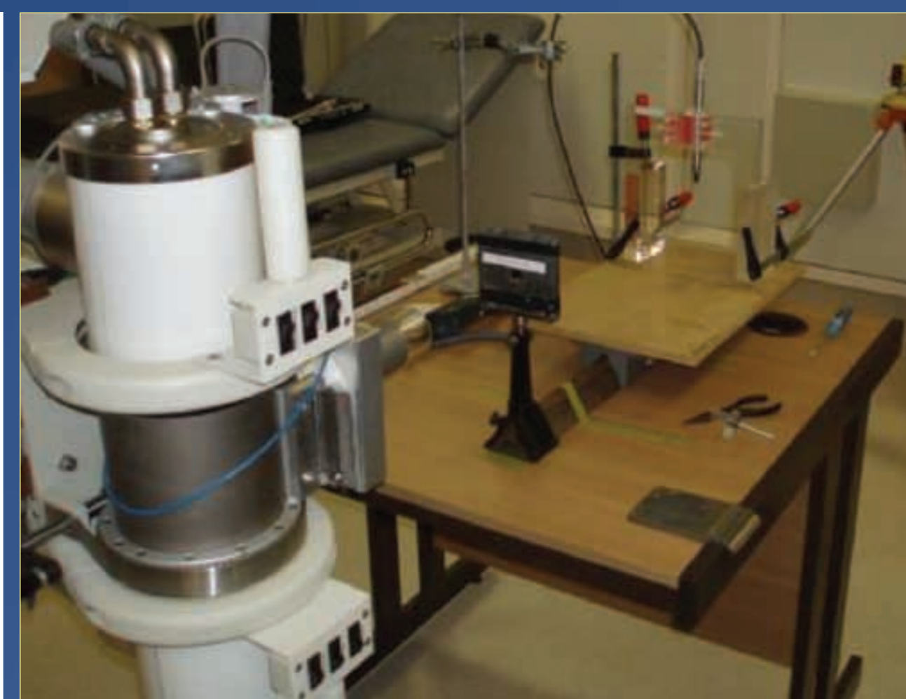
Measurement of kV beam quality (HVL)
