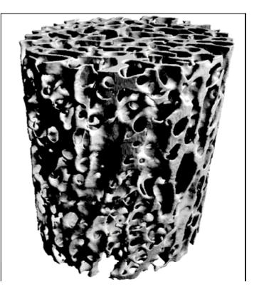
Trabecular bone specimen of a human femoral neck scanned at a resolution of 22 micron
