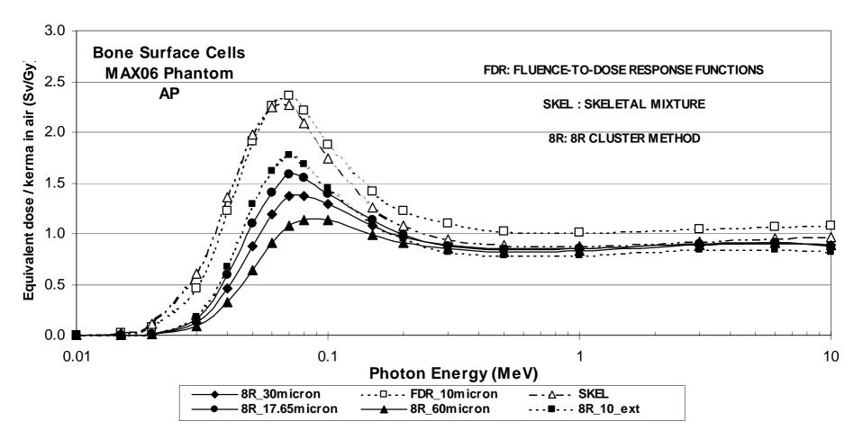
**BSC** equivalent dose per air kerma free-in-air as a function of the photon energy for AP-incidence in the MAX06 phantom for different dosimetric methods
