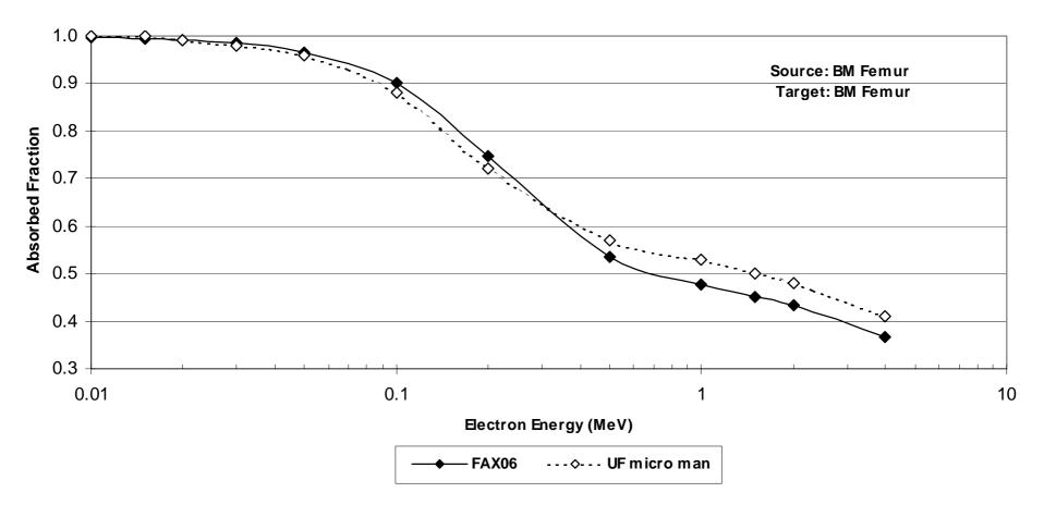
Absorbed fractions for bone marrow from beta emitters uniformly distributed in bone marrow of the femurs of the FAX06 phantom and the femoral head of the "UF micro man" as a function of the electron energy.
