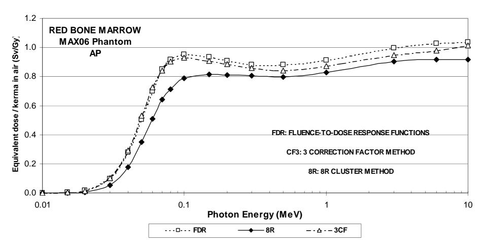
**RBM** equivalent dose per air kerma free-in-air as a function of the photon energy for AP-incidence in the MAX06 phantom for different dosimetric methods
