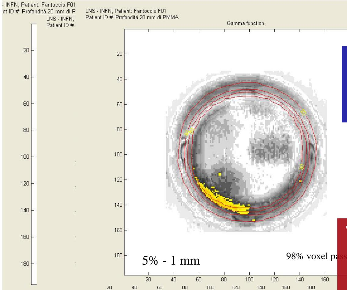
Gamma function distribution is not uniform, the values fails criteria are focused around 90 % isodose level
