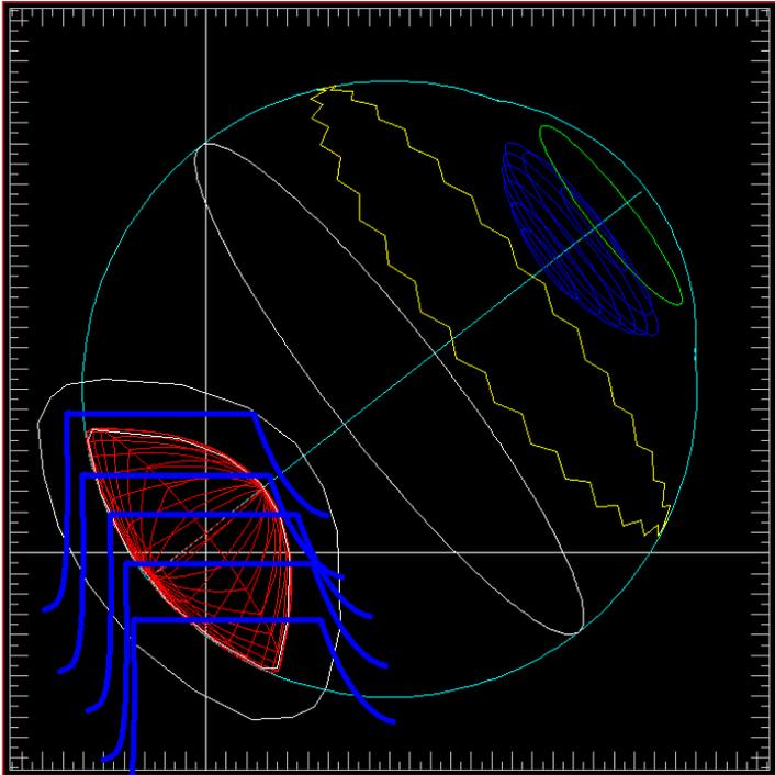
**Eyeplan reconstructs eye dose distribution so that isodose 90% enclose totally PTV, with a security Margin of 2,5 mm**
