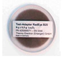
50 mm diameter, 3 mm height (acrylic glass housing) 40 mm diameter, 1 mm height (Lu<sub>2</sub>O<sub>3</sub> ceramics inlet) Typical net count rate for RadEye B20: 6 cps
