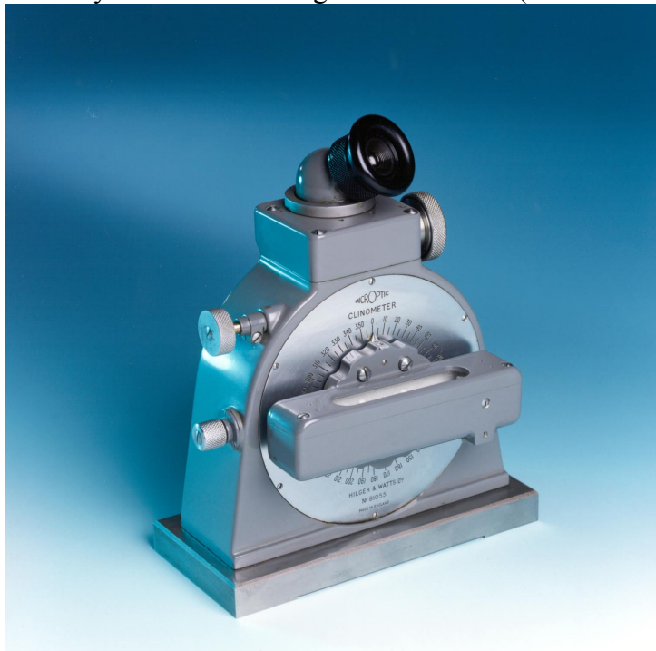
Figure 1 A Clinometer (5 second graduations)
