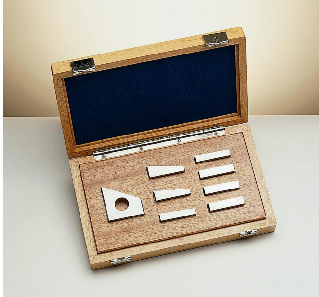
Figure 2 A Set of Hilger type Angle Gauges (picture courtesy of Taylor Hobson Limited)
