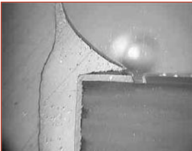
Fillet lifting and tearing during wave soldering
