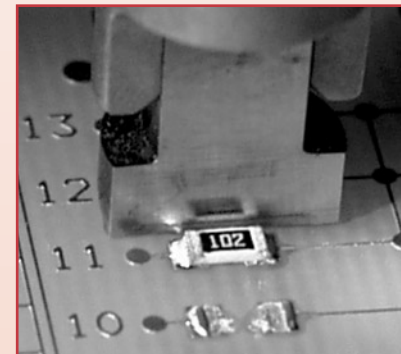
Test set up showing one tested joint and one joint before test.
