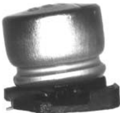
Electrolytic capacitor after lead-free soldering showing significant expansion in top and bottom of casing.
