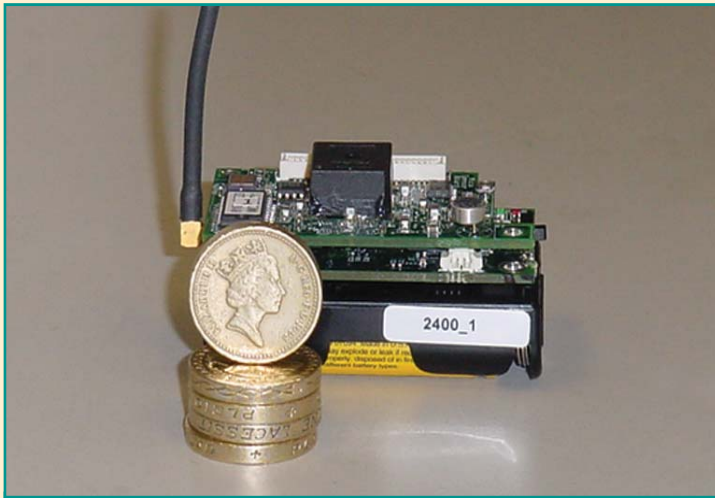
MicaZ node - part of the NPL wireless sensor network testbed
