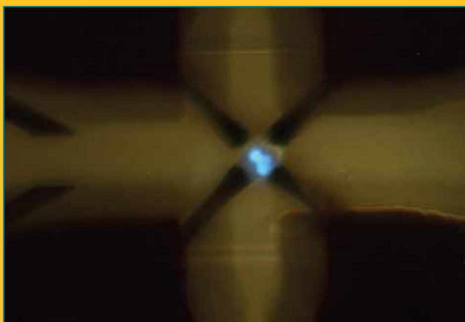
Figure 3: Three cells held in cage element and stained with Hoechst stain to visualise via fluorescent microscopy.
