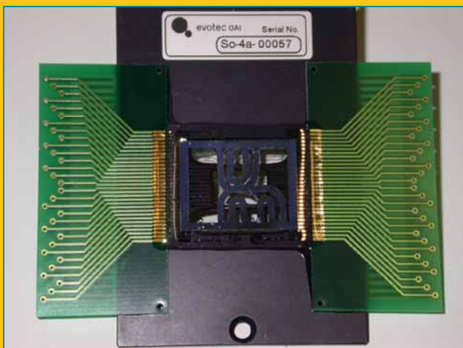
Figure 1: Dielectrophoresis chip for single cell analysis and separation
