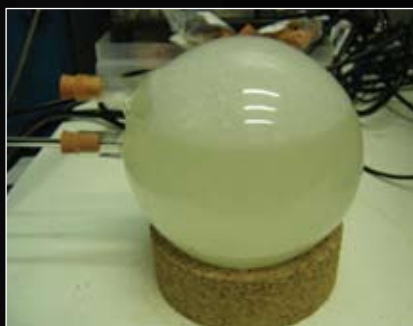
A reference target for calibrating MRI thermometry
