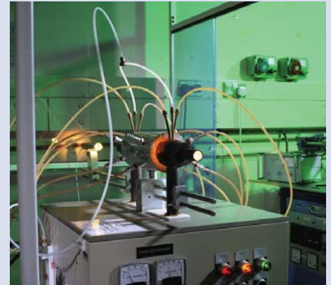
A high temperature reference – the intensity of the light emitted from the furnace is a fixed quantity and allows calibration of both radiation thermometers and detectors.
