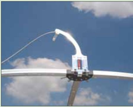
Figure 1. Picture of the nadir entrance optic in radiance orientation
