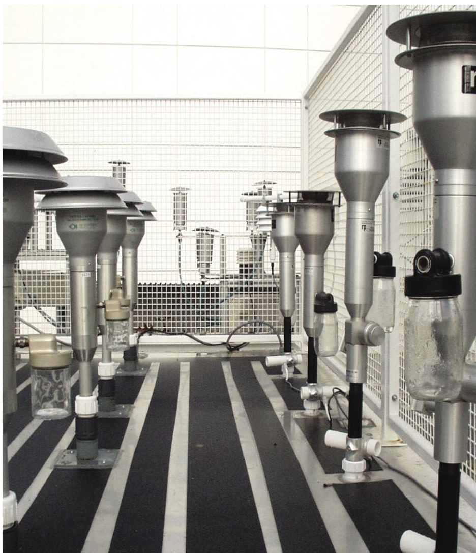
A comparative trial at NPL - sampling the air for PM10 with size selective inlets
