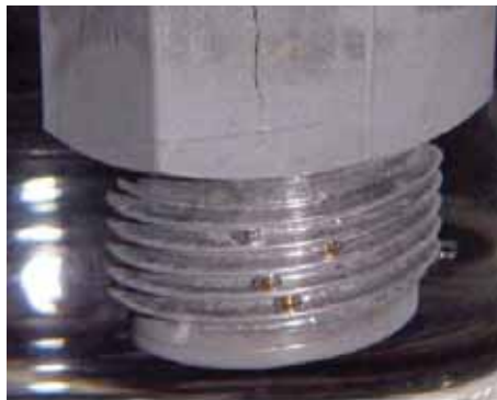
Brass adaptor in water-filled fire extinguisher. Cracks are forming in laboratory test in mercurous nitrate solution
