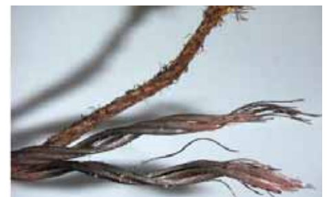
Failed wire rope
