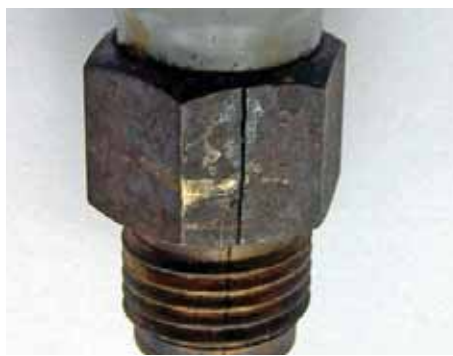
Brass adaptor in water-filled fire extinguisher. Cracks were formed in service
