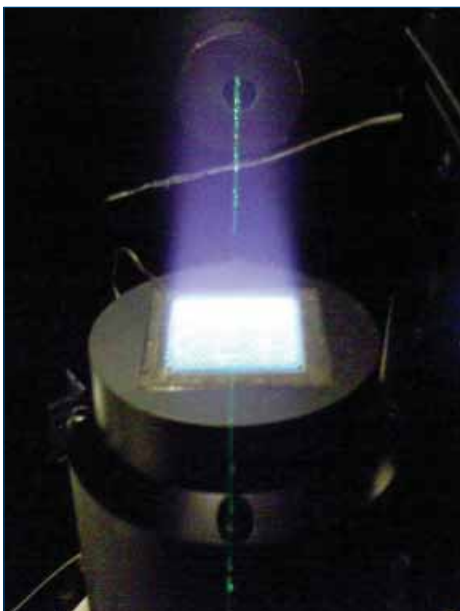
Photograph showing the Rayleigh scattering experiment in the Standard flame - a green laser beam can be seen. The portable square burner is used.
