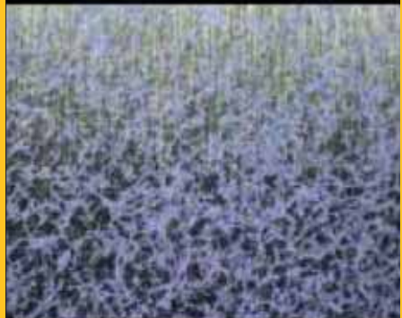
Plotting the standard deviation of each individual point with respect to a mean plane clearly shows the differences in local texture.
