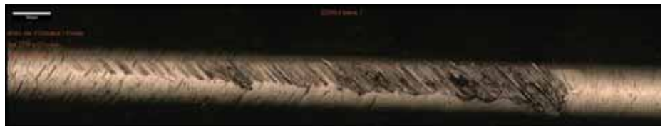
Five pass test on 316L stainless sample
