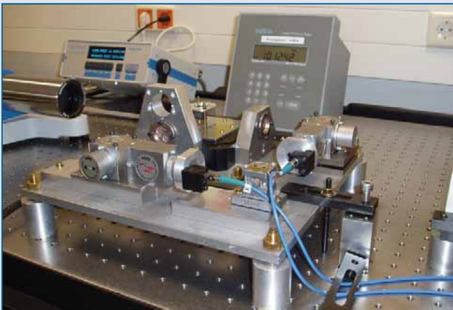
Translation stage calibration facility with interferometers for calibrating the x and y-axes and an autocollimator to measure pitch and yaw in the x-axis.
