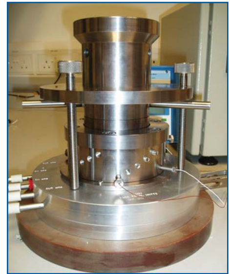
NPL apparatus for measuring thermal conductivity and heat transfer co-efficients under conditions relevant to polymer processing
