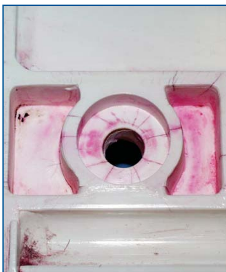
Stress induced cracking of a polymer moulding (revealed by dye penetrant inspection).
