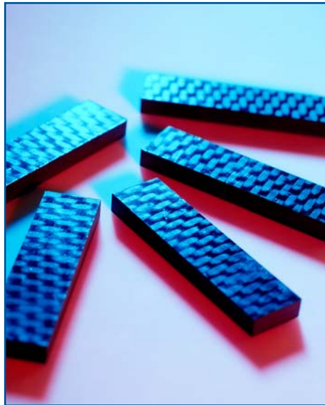
CFRP temperature reference specimens manufactured at NPL.
