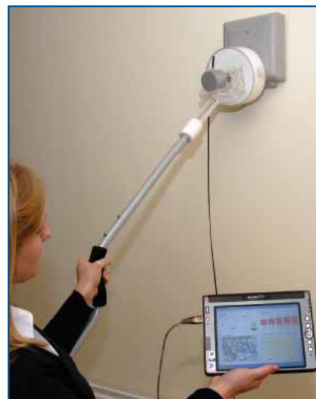
Final Instrument: Touchsafe meter developed in collaboration with IndexSAR for assessing EM radiation exposure levels close to transmitters.
