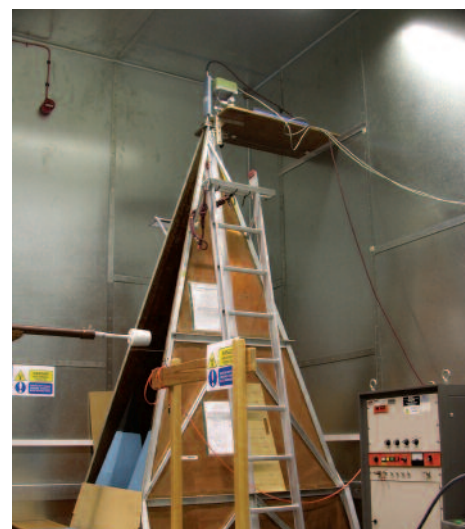
NPL Tapered TEM Cell used for calibrating field probes from 180 MHz to 2.5 GHz
