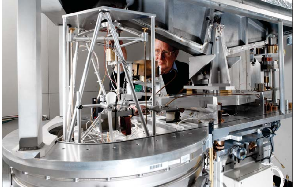
Figure 5 The Watt balance – understanding environmental vibration is vital in ensuring accurate realisation of the kilogram.
