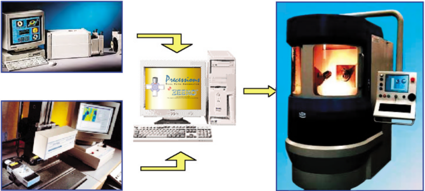
Figure 7: The Zeeko Process: from metrology to corrective polishing
