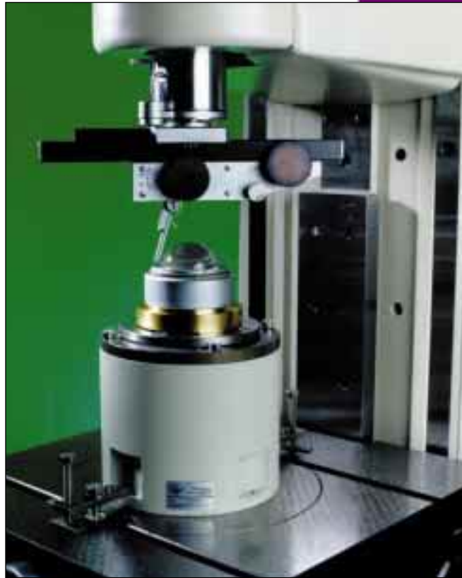
The Talyrond 73HPR roundness instrument
