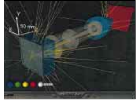
Visualisation of X-ray production using the NPL electron linear accelerator
