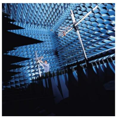
NPL fully anechoic room 9 m x 6 m x 6 m
