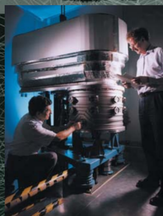
The electrical realisation of the kilogram at NPL
